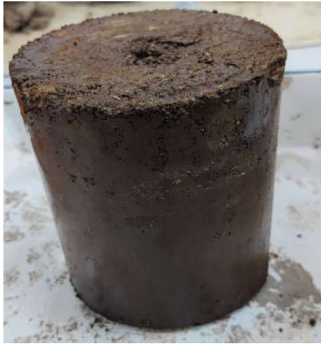
FIG.6 EXTRUDED SAMPLE AFTER COMPACTION TEST
