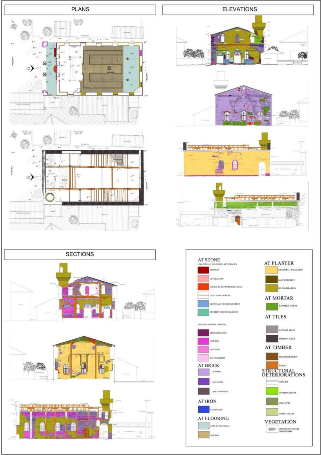
Figure 4. Materials and structural deterioration of the building (authors' archive).
