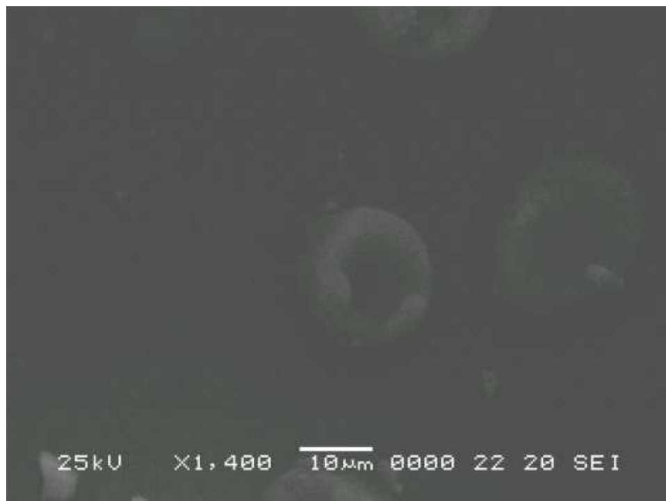
Figure 5 SEM micrographs of Plasticized Chitosan Film (CS-G30)
