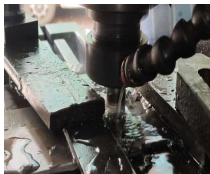
b) FSW Setup with coolant (water)
