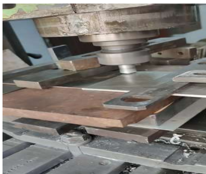
Fig. 2, a) FSW Setup without coolant
