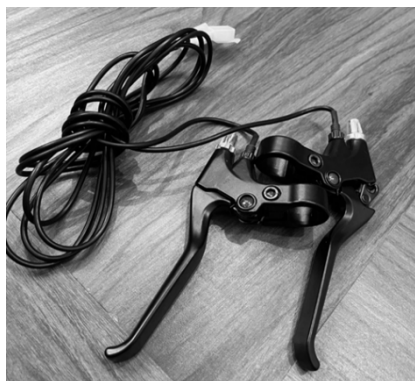
Fig.6. Electronic brake levers with cut off
