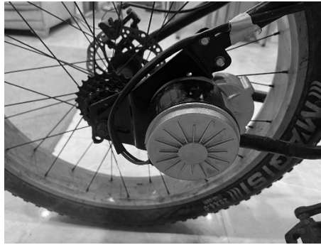
Fig.9. Motor mounted on rear stay
