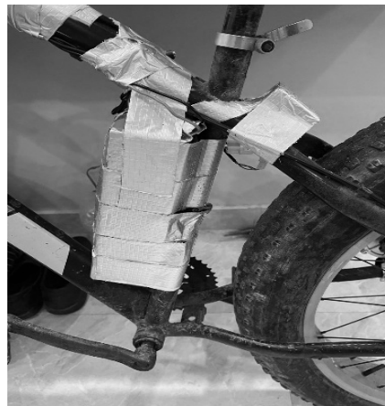
Fig.10. Prototyped battery and wiring mount
