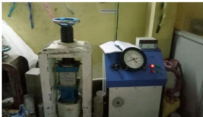
Fig -1: Cube Compressive Strength – Experimental set up
