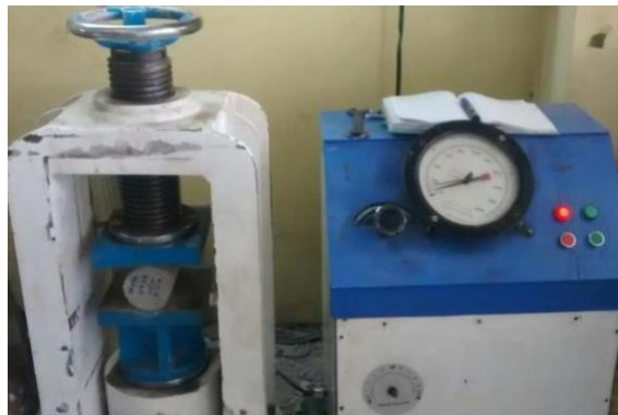
Fig -2: Split tensile Strength – Experimental set up
